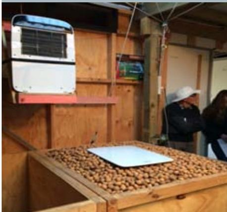
Dehumidifiers are more efficient at higher temperatures and lose their efficiency at lower temperatures so a domestic oil column heater is used to keep that drying room at 20 degrees or better. This year the nuts stayed in the drying bins for about four days to get them to the required moisture content.
