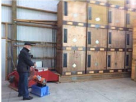
The bins have inspection holes for sampling the nuts for moisture content. Frank uses a Protie meter to measure the moisture level in the minced shell and kernel. The nuts this year took 60 hours to dry to a 9% moisture level.
