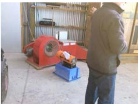
Warm air flows up through the bins drying the nuts. Sensors in the bins monitor the humidity and temperature with heating turned off at 40 degrees. The airflow through the bins is strong enough to float a sheet of ply sitting on the bins.
